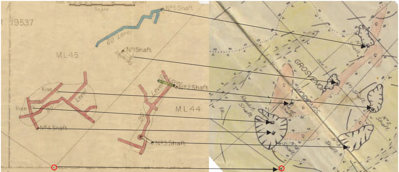
Figure 3.16 Extract of Grosvenor workings from 'Geological Map of Leadville – N.S.W' by The Zinc Corporation Ltd, 1948. In GS1948/008 (DIGS Ref. D00586920) correlation to Grosvenor plan DIGS Ref. D003796380
