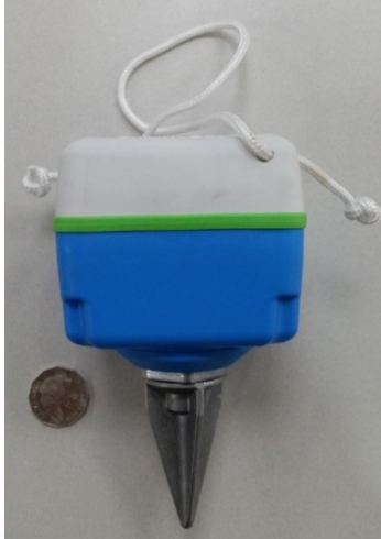
Figure 2 A geophone node that records ground vibrations.
