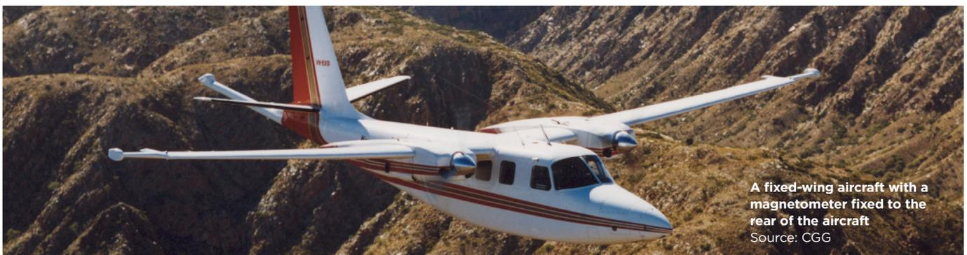
A fixed-wing aircraft with a magnetometer fixed to the rear of the aircraft
