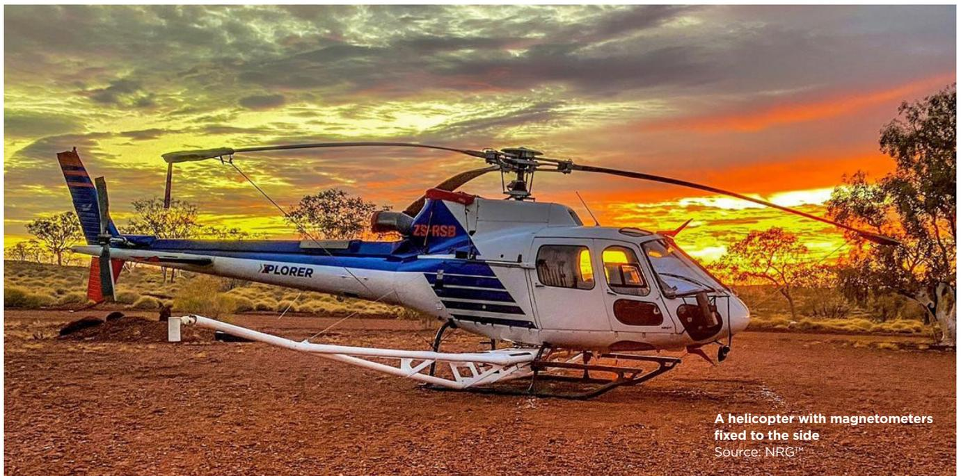
A helicopter with magnetometers fixed to the side
